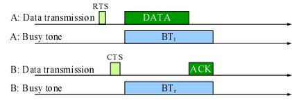
Fig. 7. The Time Diagram of BT-DMAC
